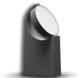
Mimosa Pedestal Antracit 1x7W 27K 8719514477292 ↔ 120 ↗ 120 ↓ 250 mm LED 7 W, 630 lm @ 2700 K
