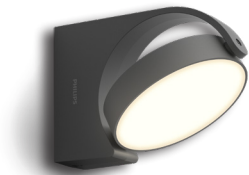
Mimosa Wall Antracit 1x7W 27K 8719514477254 ↔ 120 ↗ 117 ↓ 171 mm LED 7 W, 630 lm @ 2700 K
